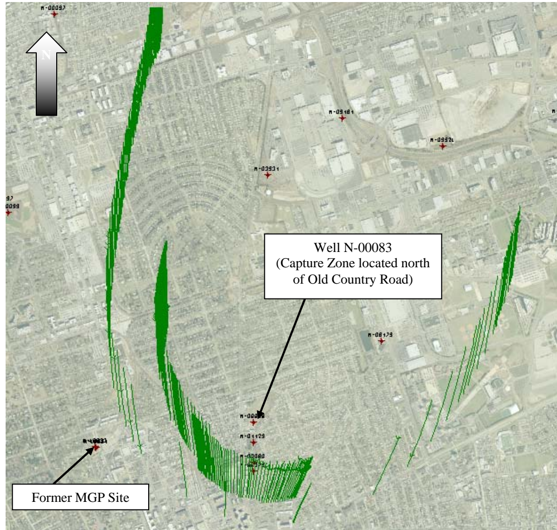
FIGURE 5-5 CAPTURE ZONE FOR WELL N-00083 MAXIMUM PUMPAGE SCENARIO
