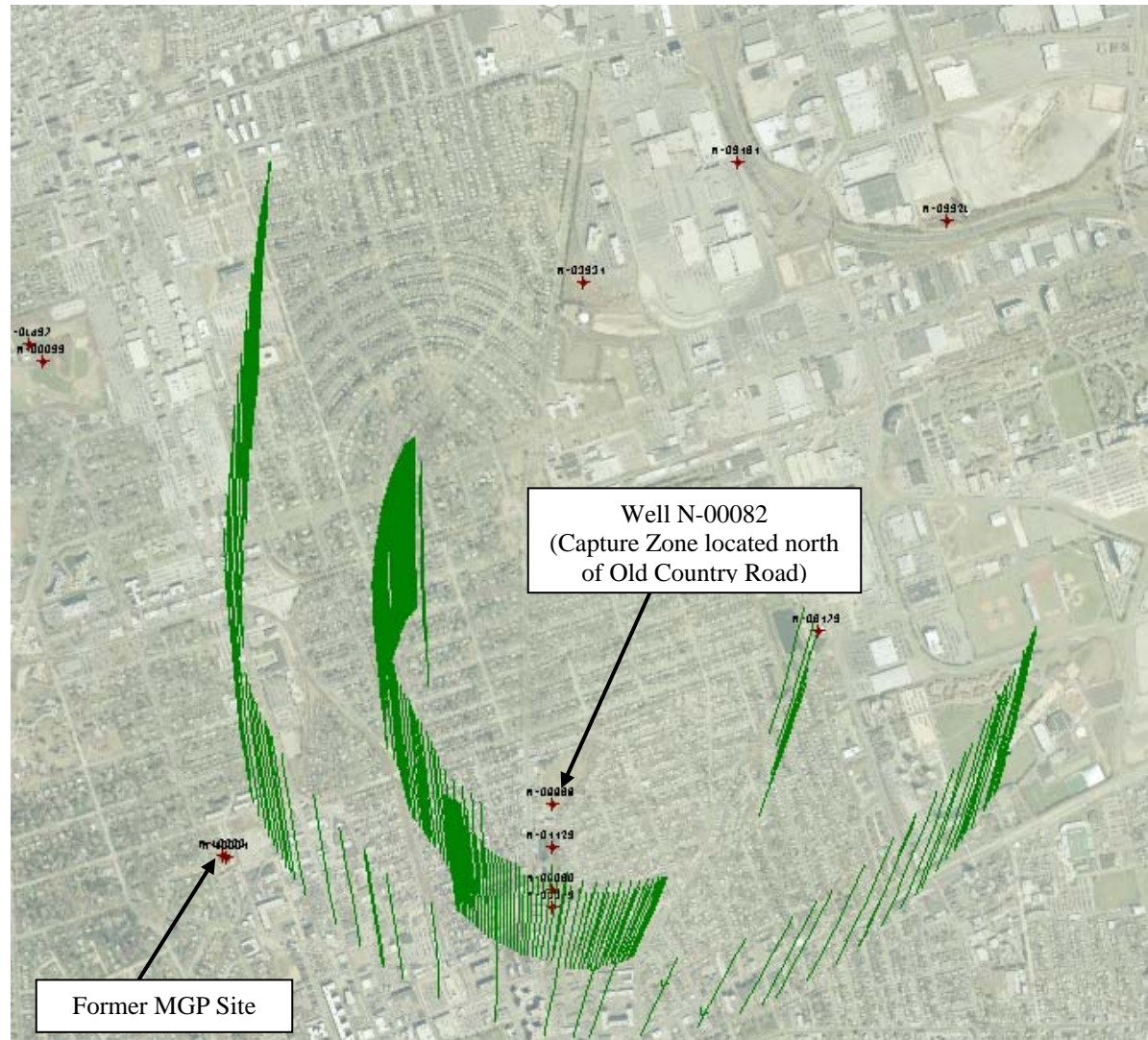
FIGURE 5-4 CAPTURE ZONE FOR WELL N-00082 MAXIMUM PUMPAGE SCENARIO
