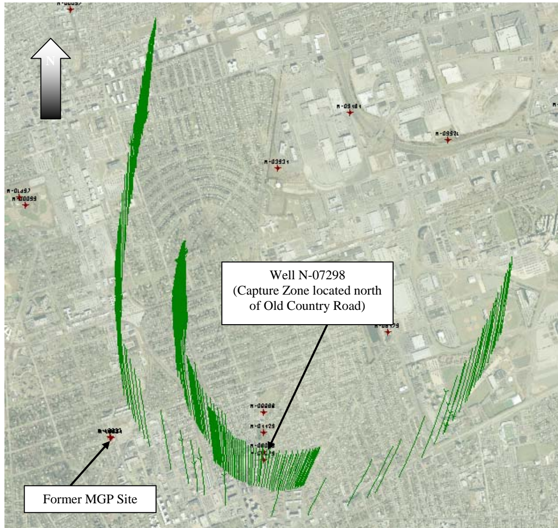
FIGURE 5-7 CAPTURE ZONE FOR WELL N-07298 MAXIMUM PUMPAGE SCENARIO
